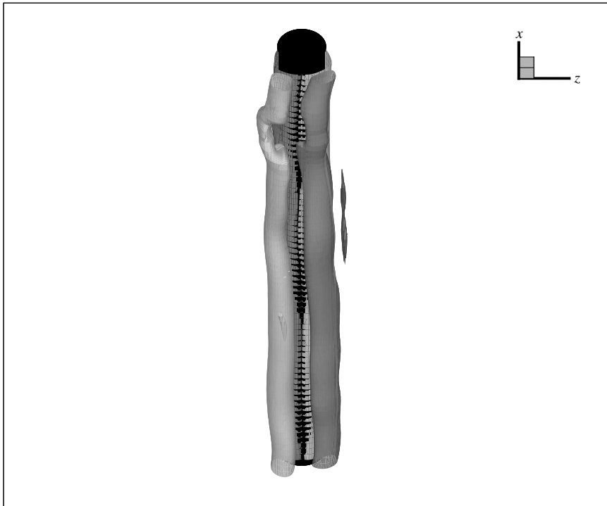
FIGURE 21. Instantaneous three-dimensional view of the vorticity \omega_y near the cylinder, at the phase t_p = 0 of the 141st cycle. Regime F, KC = 8.5 , \beta = 20 , Re = 170 .
